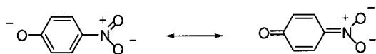
FIGURE 5. Resonance contributors of p -nitrophenolate ion, showing involvement of the nitro group in charge delocalization that gives rise to the N-15 isotope effect.
